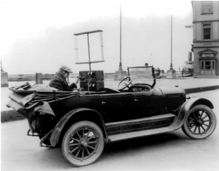
First Mobile Radio Telephone 1924
